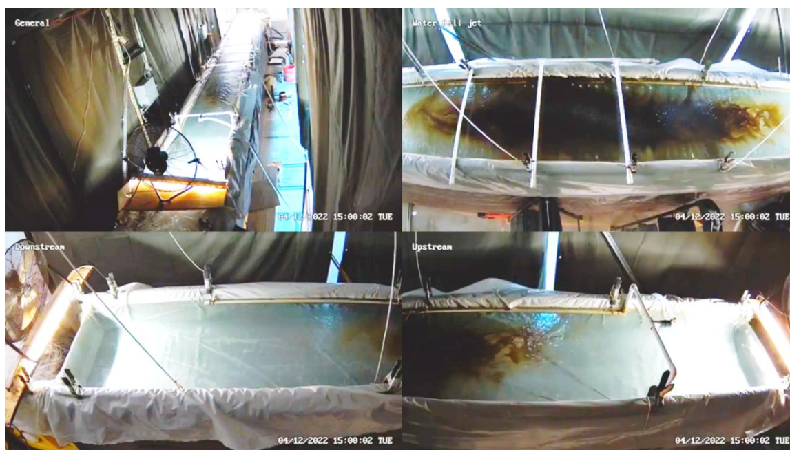
Fig. 2 The photos taken by the CCTV monitoring camera show the movement of surface oil.
